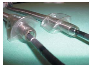
Figure 1. The Recommended Size of the Gap between the Tube and the Fiberoptic.
